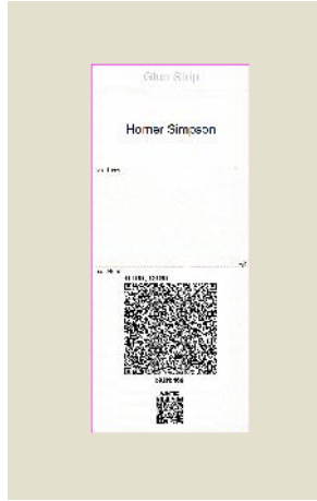
Fig. 2: Audit ballot. The audit information is printed in the barcode in the lowest part of the ballot
